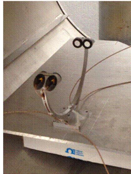
**Figure 2. Mars Acoustic Anemometer in a test chamber at Ball Aerospace**
