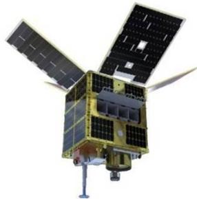
Figure 3. Enhanced Microsat with CubeSat Deployers
