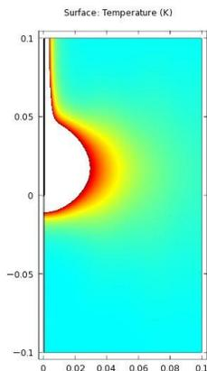
radially with processing time. The diameter of the heated volume will be a function of the microwave frequency and time.
