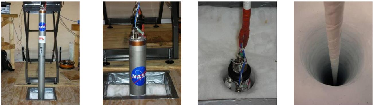
Figure 1: A 7 cm diameter thermal drill descends into the Greenland ice cap returning meltwater for analysis through an aerogel-insulated tether. In the final frame, the drill is 47 m below the surface (images from JPL).
