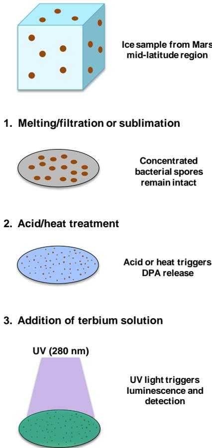
Fig. 2. Schematic of experimental design
