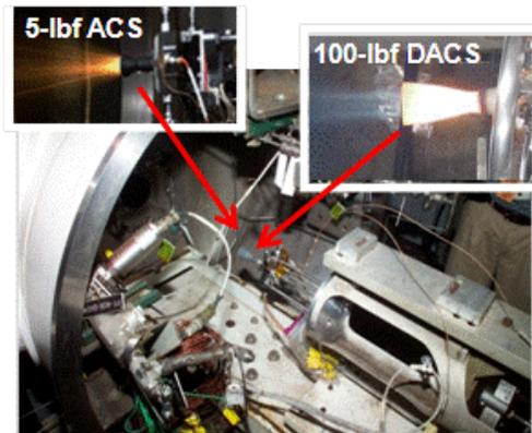
Figure 1: Successful Hot-Fire Evaluation of Heritage MDA Thrusters at WSTF in Vacuum Chamber
