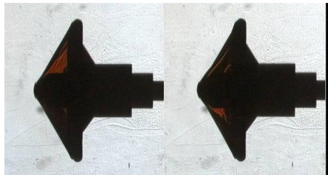
Fig. 3. Hypersonic wind tunnel testing of thin film ballute articles provides flow field and deformation data for CFD and aeroelastic model validation.
