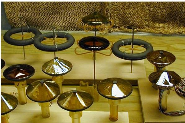
Fig. 2. Several thin film and free flying ballute wind tunnel models of various configurations were constructed and tested at NASA Langley.
