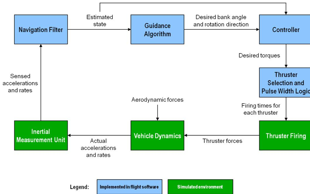
Figure 1. Flightworthy aerocapture GN&C software has been developed and tested in real-time, hardware in the loop simulations.
