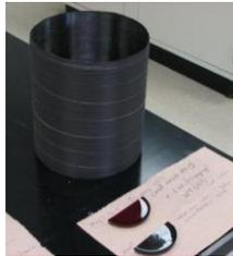
Wound and cured IL epoxy/carbon composite
