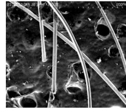
SEM of carbon fibers made in the laboratory from IL-processed rayon precursor
