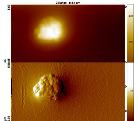
Figure 2: A topographic (top) and phase (bottom) MIDAS scan of a micron sized calcite particle.
