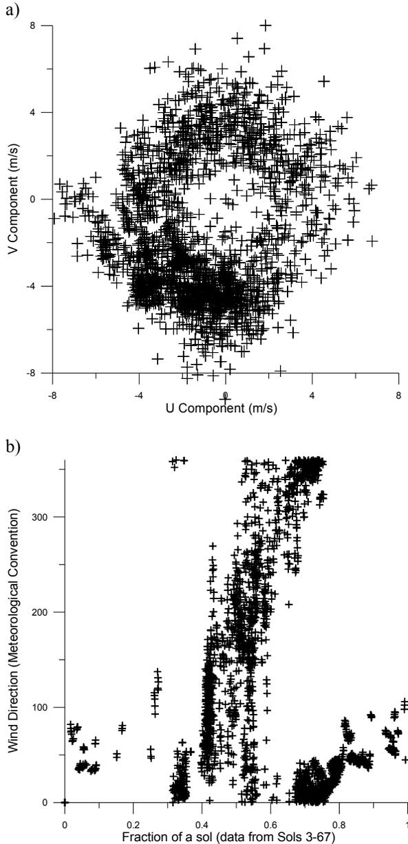
Figure 2. Preliminary telltale wind data from Sols 3-67. a) U and V components, b) Wind direction vs time of sol. (LMST)
