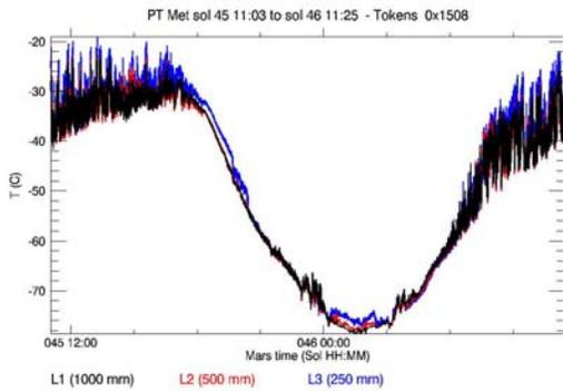
Figure 3: The preliminary diurnal cycle of temperature from the Phoenix thermocouples (sols 45-46) with heights given in meters above the lander deck.
