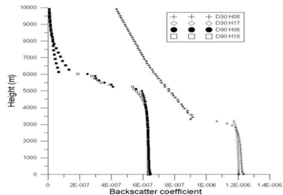
Figure 2: LIDAR backscatter determined from ABL model at two times on sols with and without the presence of dust above the boundary-layer.
