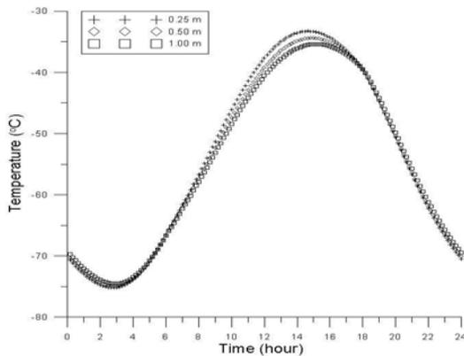
Figure 4: ABL model at 0.25, 0.5 and 1 m above the lander deck for optical depth of 0.3.
