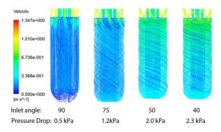
Figure 1: A series of CFD simulations of a 4 MWt space molten salt reactor. Different angles of inlet pipes were tested to minimize stagnant fuel.
