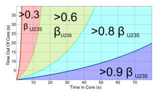
Figure 2: Regions of  $\beta_{eff}$  in terms of equivalent solid fuel  $\beta_{U-235}$  for a molten salt reactor fueled with U-235 as a function of time in and out of the core.
