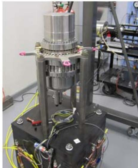
**Figure 2.** Single Convertor Attached to Large Mass
