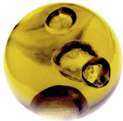
Figure 1 Blowing inside a sphere of resin in microgravity. What could be the future's space souvenir?
