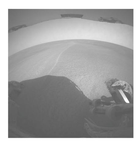
On B-446, 50 meters of blind driving made only 2 meters progress, burying the wheels. Recovery time: 5 weeks.
