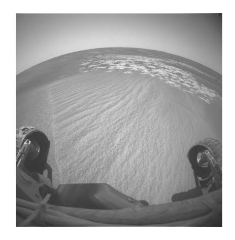
On B-603, 5 meters of blind driving made 4 meters progress (stopped by Visodom with 44% slip). Recovery time: 1 day.
