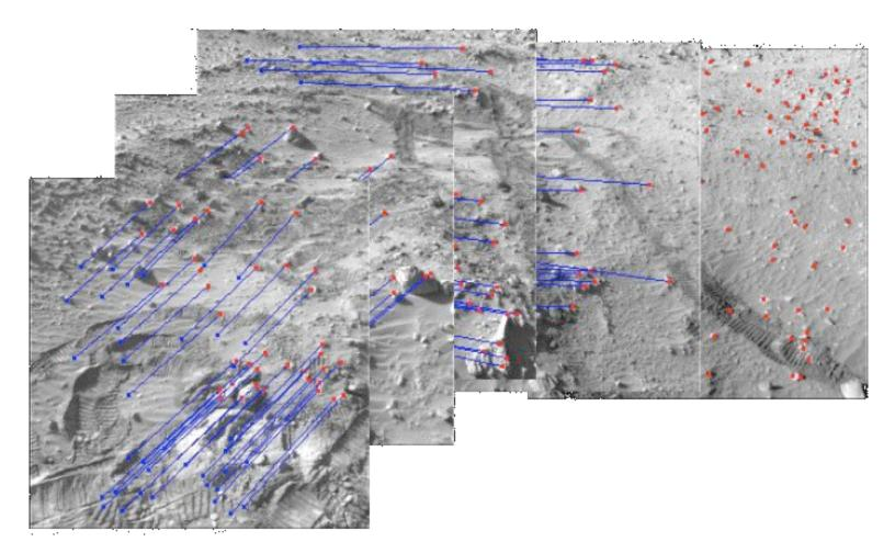
VisOdom enables precise position estimates, even in the presence of slip, and enables Slip Checks and Keep-out zone reactive checks
