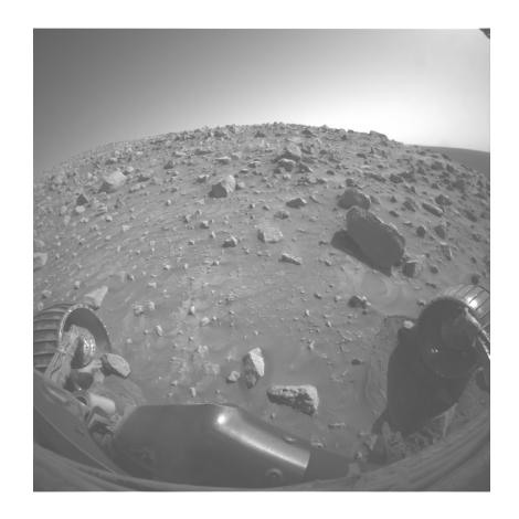
On A-454, Spirit detected 90% slip and stopped with rocks poised to enter the wheel. Recovery time: 1 day.
