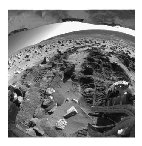
On A-345, Spirit stalled because a potato-sized rock had gotten wedged inside a wheel. Recovery time: 1 week.
