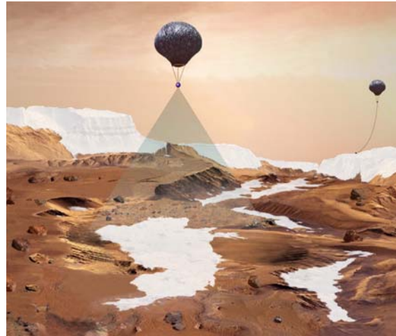
Figure 1. Balloon sampling may enhance our ability to carry out exploration over rugged landscapes on Mars such as the polar caps and erg. Under development for solar driven Montgolfiere balloons is the ability to approach the surface for rapid acquisition with a “touch-and-go” sampler.
