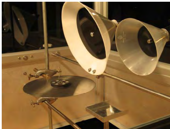
Fig. 5: Protection caps being lifted off the caltarget and a calibration plate for the experiment
