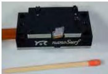
Fig. 1. The electromagnetic scanner head (black anodized) with the micro-fabricated sensor chip mounted in front of it.
