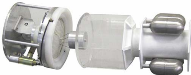
Figure 3: WEB docking system breadboard hardware. Lander (left) near capture with return spacecraft
