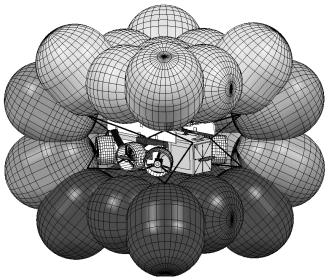
Figure 1: Bottom isometric view of pallet lander.
