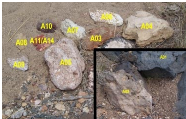
Figure 1 - Samples measured in the field with both the LIBS and reflectance instruments. Sample A05 is approximately eight inches long.
