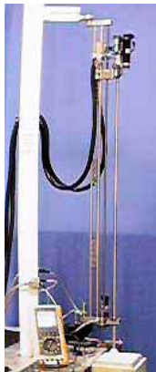
Figure 1: The 1 Meter Deep Drilling SATM Prototype
