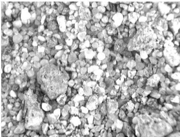
Figure 3. Monochrome version of FIDO Color Microscopic Imager [6] data from May 2001 field test, showing natural soil illuminated by skylight (target in shadow). View is about 13 mm across, 20 microns/pixel, taken at f/10 .
