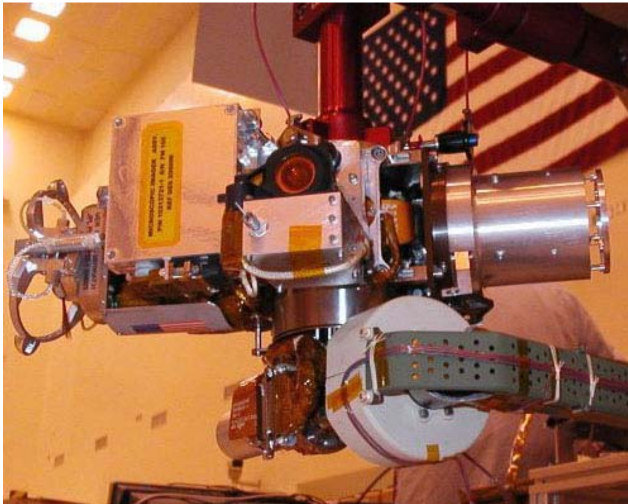
Figure 1. IDD instrument turret during MER 2 testing. RAT at left, MI at center, APXS at right (Mössbauer spectrometer not visible). MI dust cover is shown closed, with contact sensor to lower left.
