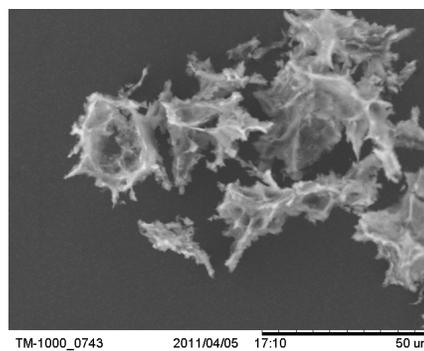
Figure 1: SEM image of vacuum-dried powder, no isolated grains can be distinguished even at a resolution of ~5 μm.
