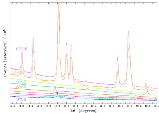
Figure 3: Crystallisation sequence of amorphous  $\text{Mg}_{(0.5)}\text{Ca}_{(0.5)}\text{SiO}_3$
