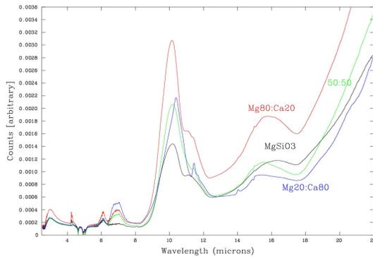
Figure 2: FTIR spectra of sample compositions  $x = 0, 0.2, 0.5, 0.8, 1$
