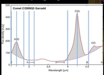
Continuum subtraction ratio of CO<sub>2</sub> to H<sub>2</sub>O emissions, using eight narrow band spectral filters (indicated by the blue vertical lines)
