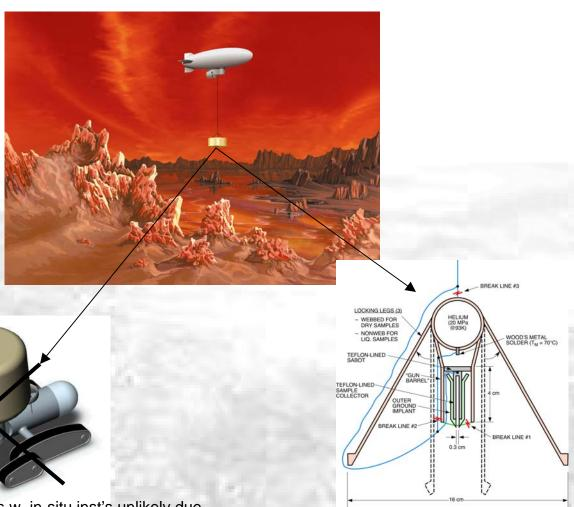
Passive/Mobile sondes w. in-situ inst's unlikely due to power (high heat) and cleaning/purging rqrs which will rqr batteries/purge gas components not compatible w. volume constraints of sonde
