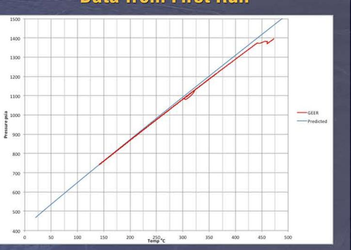
Blue line is predicted behavior. Red line is actual data. The pressure anomaly at 437 C and 130 psi is very intriguing. Testing to date suggests data is a real condition and not instrumentation anomaly.
