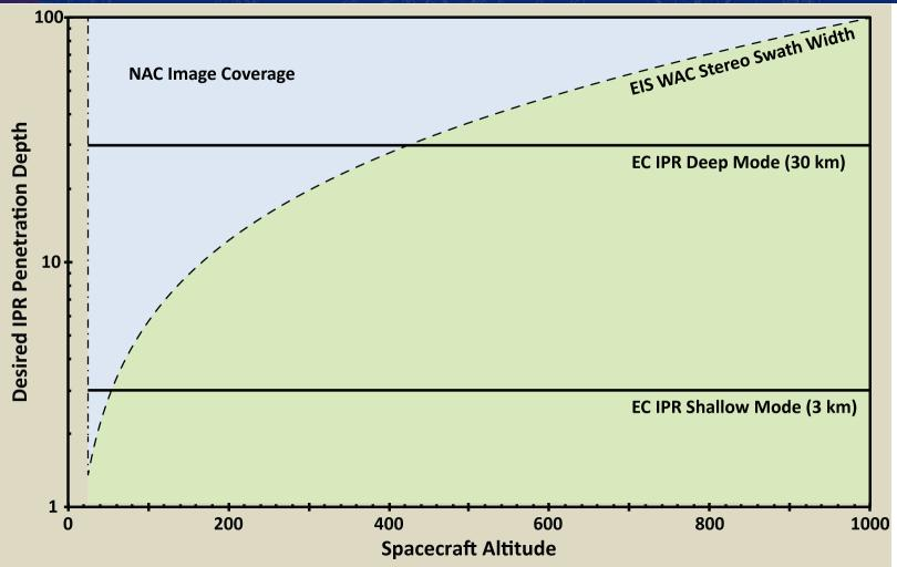
Maximum penetration depth d (km) for which EIS characterizes surface clutter as a function of s/c altitude (km) compared to penetration depths of EC IPR deep and shallow modes (n=1.78).
