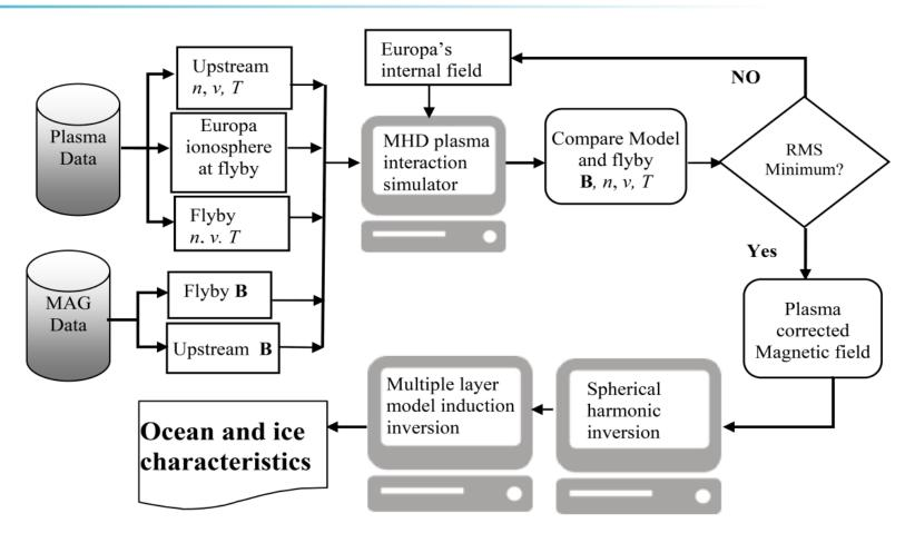
The MHD plasma interaction simulator, fed by the mag and plasma data, is key for isolating the induced magnetic field. The aggregated plasma-corrected Europa mag data set is decomposed into the primary external field and seven wave frequencies from which ocean and ice characteristics are derived.
