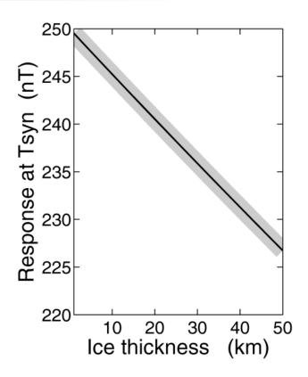
The induction response to the expected 250 nT (Bz) field at 11.2-hr period is linearly related to the ice shell thickness when d  $<< R_E$ . The shaded region shows the expected ICEMAG accuracy of  $\pm 1.5$  nT.
