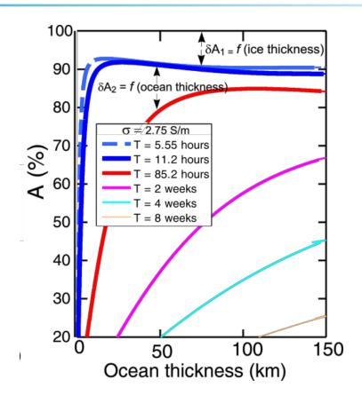
Induction response (efficiency), A, at multiple frequencies allows a unique determination of the thickness of the ice shell, and further constrains the ocean depth.
