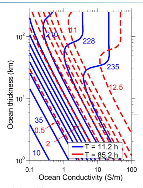
Induced field (in nT) at the surface of Europa in response to the 11.2-hr (blue, solid lines) and 85.2-hr waves (red, dashed lines) show that response at multiple frequencies can uniquely determine ocean parameters.
