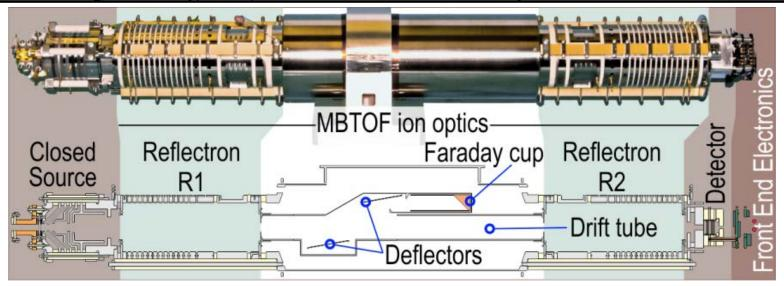
MBTOF cross section and photo of the third-generation instrument identifying the arrangement of the major components
