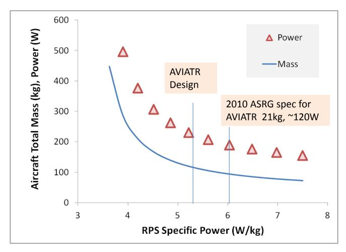
Specific Power is enabling for this mission! Thermoelectrics have much lower performance by this metric: MMRTG performance (~2.8W/kg) at the time of the study is not even on this chart!
