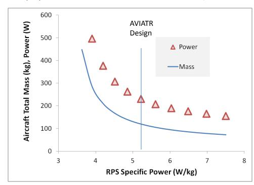
Reality check – empirical scaling, Lorenz, Journal of Aircraft, 2002 says V~11m<sup>0.8</sup>V<sup>0.9</sup>(g/g<sub>e</sub>)( $\rho_e/\rho$ ) - for 115 kg at 6.2 m/s is ~192W
