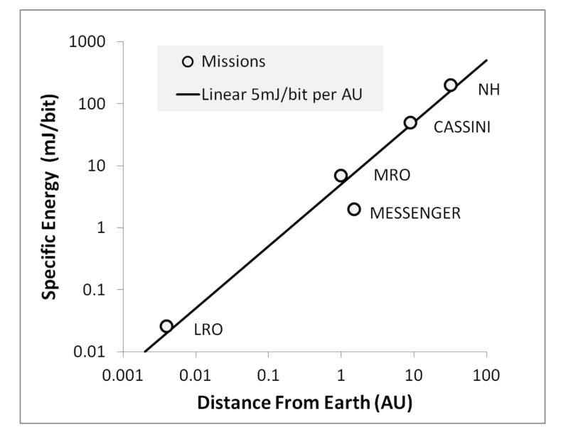
Spacecraft with High-Gain Antennas. Surprisingly linear dependence of specific energy with distance
