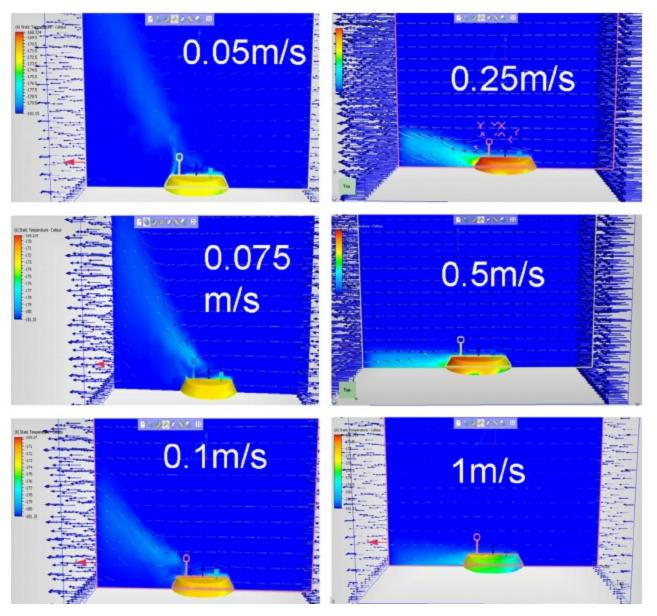
Thermal plume leans over with increased windspeed — for 1kW heat output, a short (~1m) mast is adequate for winds >0.1m/s
