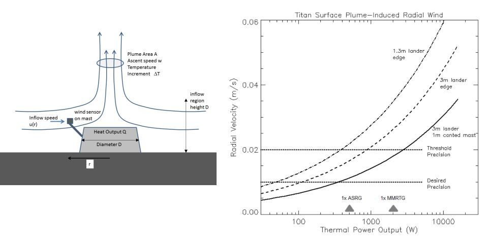
Lander-induced thermal perturbations become more severe at higher heat loads/densities – even generate a local wind. Can be mitigated with canted meteorology mast (again, mitigations to non-preferred RPS options are possible, but are crippling in a cost-constrained mission scenario.)
