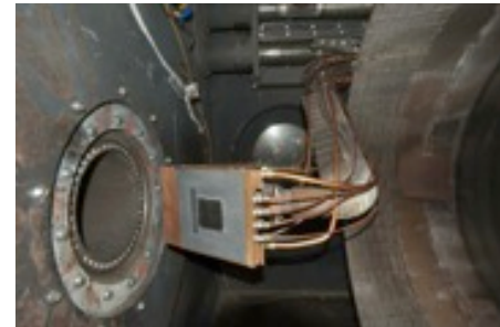
Carbon fabric arcjet testing (2012)
