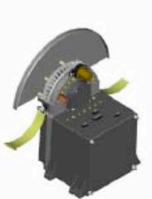
Pluto Energetic Particle Spectrometer Science Investigation (PEPSSI). CBE mass 1.41 kg, power 2.32 W
