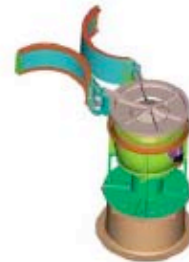
Solar Wind Around Pluto (SWAP), CBE mass 2.94 kg, power 2.25 W
