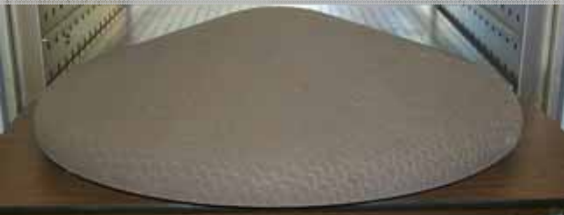
1-m SRAM-20 aeroshell test at Solar Tower
