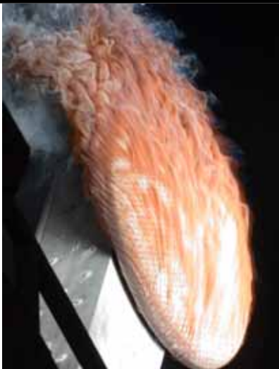
1-m SRAM-20 aeroshell test at Solar Tower
