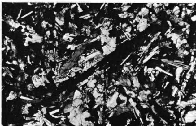
Fig. 4.37. Photomicrographs of typical lunar mare basalt textural varieties. (a) Porphyritic, (b) Ophitic and (c) Intersertal. The longest dimension of each photo is 3.1 mm (NASA Photos S-70-49563, S-70-49438, S-70-48984).
