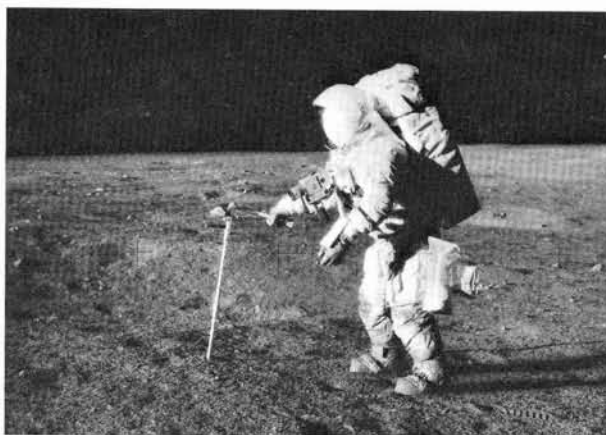
Fig. 6.4. Sampling the lunar soil with a drive tube during the Apollo 12 mission (NASA Photo AS12-49-7286).
