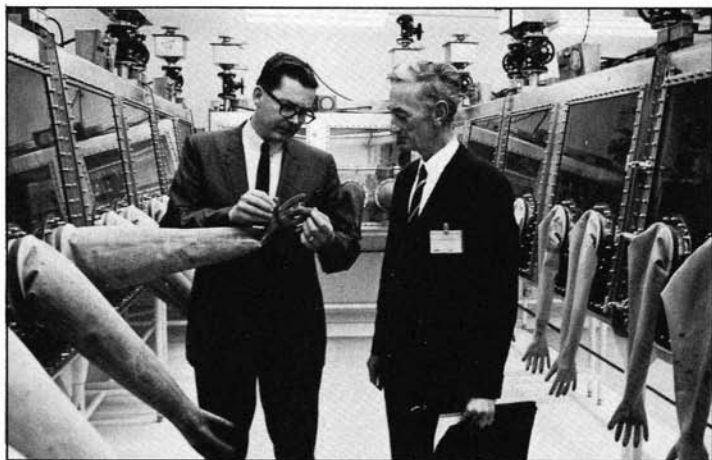
Photo 41. Author (left) shows Prof. Wolf von Engelhardt of the University of Tubingen, West Germany, details of the two-way biological barrier cabinetry in which the lunar samples will be examined in a dry nitrogen atmosphere. (NASA photograph S-67-45452)
