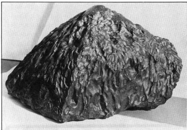
Photo 2. The Rosebud, Texas, stony meteorite (chondrite) showing a well-developed ablation surface due to heating by friction with the atmosphere during entry at high velocity. Maximum dimension is approximately 40 centimeters. (Photograph by the author)
