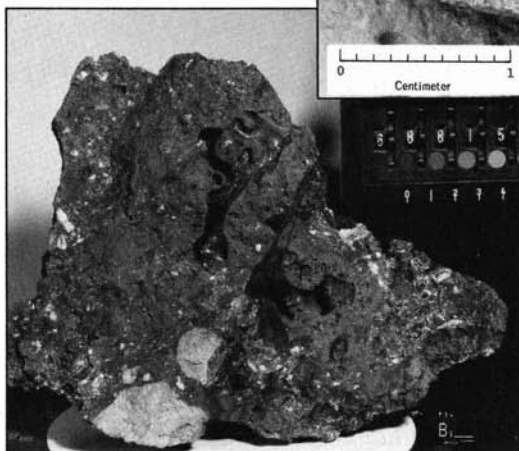
Photo 51. Glassy impact melt-breccia collected at the Apollo 16 landing site. This rock consists of many fragments with different grain sizes and textures held together by glassy material formed by meteoroid impact. Scale (right) is in centimeters. (NASA photograph S-72-37155)
