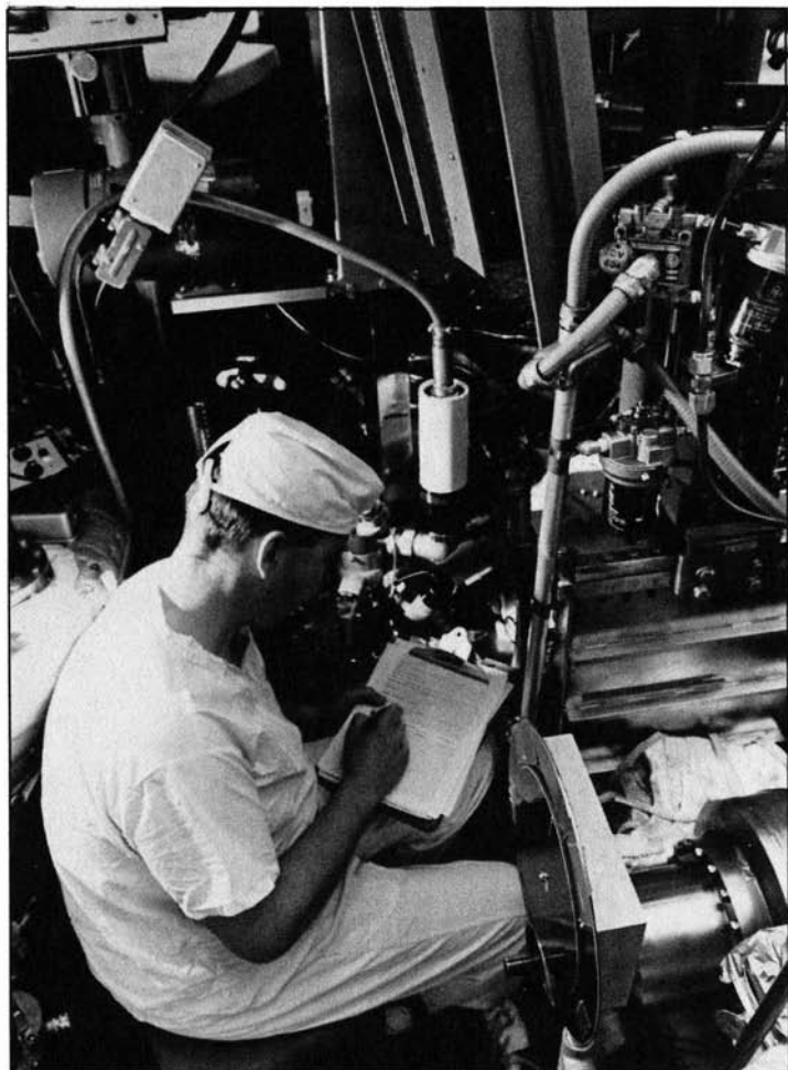
Photo 52. The author noting observations on an Apollo 11 rock sample at the main observer's port on the main vacuum system where the lunar samples were first opened. (NASA photograph S-69-29689)
