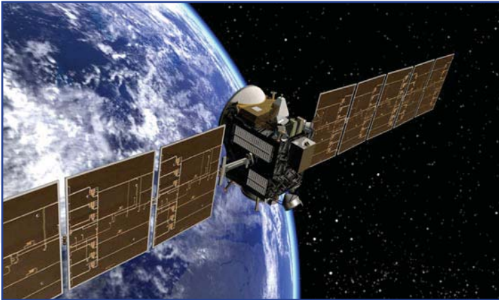
The Dawn spacecraft, illustrated in this artist's concept, is propelled by ion engines. Credit: NASA/JPL.
