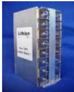
Figure 3: Prototype 25 A-hr, 28-V lithium-ion battery selected for Mars 2001 Lander http://www.grc.nasa.gov/WWW/RT1999/5000/5420manzo.html
