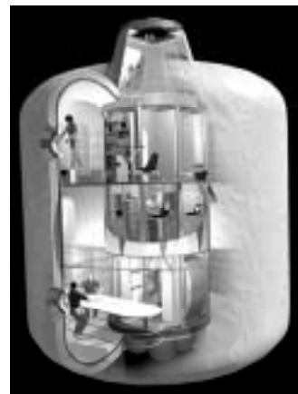
Figure 2-4: Cutaway view of the Transhab.
