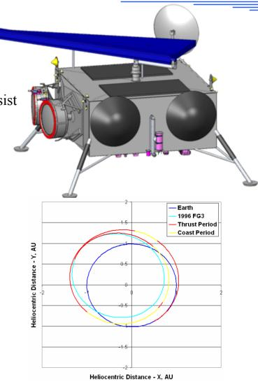
Multi-body sample return is enabled using electric propulsion
