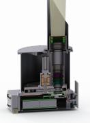
MapCam provides narrow angle OpNav, performs filter photometry, maps the surface, and images the sample site
