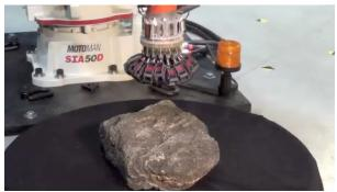
Testing of microspine gripper prototype
