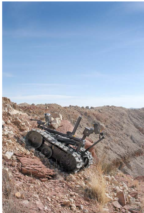
Fig. 2. Field mobility test at Meteor Crater of a terrestrial precursor of Lunar Surface Explorer. This design takes advantage of heritage developed by Foster-Miller for their Talon-series of rovers.
