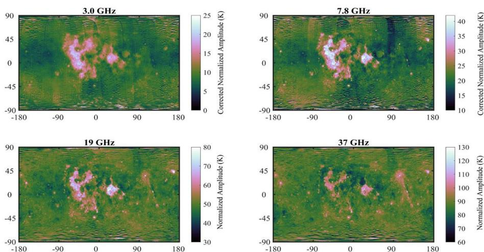
**Figure 1.** Global brightness temperature amplitudes at all Chang'E-2 frequencies after a time of day correction and latitudinal normalization plotted at 1/4 degree resolution.
