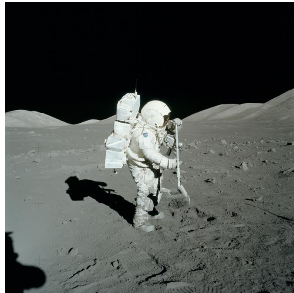
Figure 2. Jack Schmitt sampling regolith on Apollo 17 . Important geotechnical parameters can be obtained from similar crew activities on Artemis III if the forces applied to the tools can be measured, for example by adding strain gauges to the rake handle. Much effort was taken during Apollo to obtain samples of pristine regolith. For ISRU, the nature of disturbed regolith is also important to characterize.
