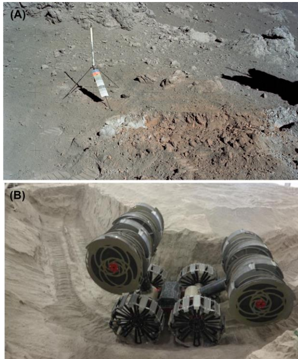
Figure 1. (A) Apollo 17 image AS17-127-20990 showing that vertical walls ~10 cm tall can be made in lunar regolith. (B) NASA JSC RASSOR vehicle trenching ~1 m into BP-1 lunar regolith simulant [4]. Will such a deep trench with vertical walls really be possible on the Moon?
