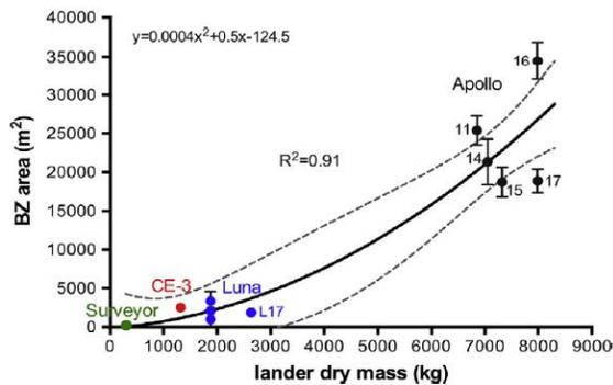
**Fig. 2:** The area of the surface visibly disturbed by rocket exhaust increases quadratically with lander mass [7].
