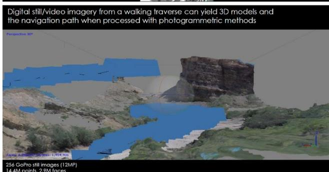
**Figure 3.** Terrestrial fieldwork increasingly uses SfM [2]. This example shows the quality of 3D model possible with optimized instruments and procedures (high resolution, continually recording, crew-mounted video camera on a walking traverse). It represents what may be achievable at the outcrop-to traverse-scale on the Moon.
